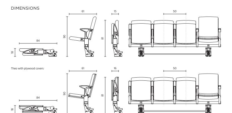
Particular dimensions can be individually adjusted to a given project. All dimensions are in centimetres.
