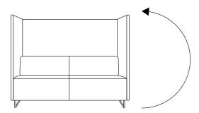
Installation and deinstallation have required turning the furniture around and laying it flat. The panels been permanently installed from the underneath and the seat has been installed with screws, they have not been connected to each other.
