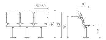
$<sup>^{\</sup>ast}$  Particular dimensions can be individually adjusted to a given project. All dimensions are in centimetres.
